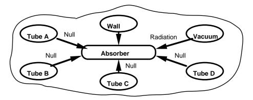
A partial view of the network representation of the collector configuration of figure 1 is shown above. The links indicate incoming transfer parameters to the context of the absorber. A radiation effect is transmitted through the vacuum to the absorbing plate. No other phenomena are currently under consideration.
