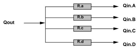
This diagram shows the equivalent electric circuit for the heat transfer model between the absorber and the water tubes. Heat transfer is by conduction. A surface pressure may also be derived due to possible expansion of the absorber as it heats up, thus exerting force on the water pipe. Transfer of heat from the pipe wall to the fluid will be via conduction and convection, depending on the spped of the water.
